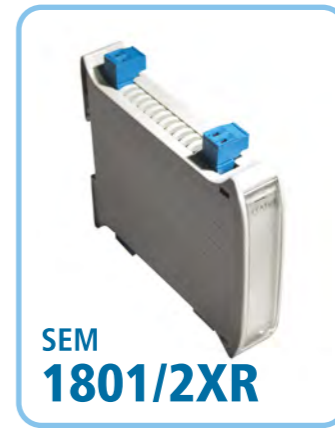
SEM 1801/2XR RTD, potentiometer, resistance transmitter; PC configuration. IS-approved.
