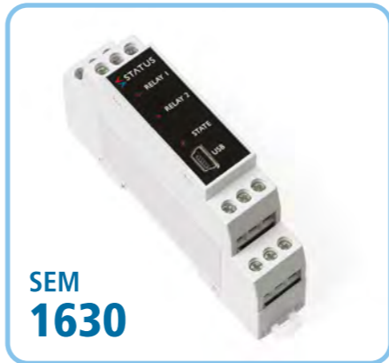
SEM 1630 RTD, thermocouple, passive mA, mV input, with 2 change-over relay outputs.
