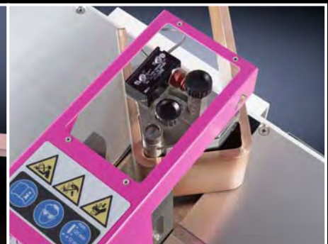
Bending a busbar
