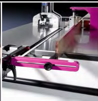
Punching busbars, pull-out measurement system
