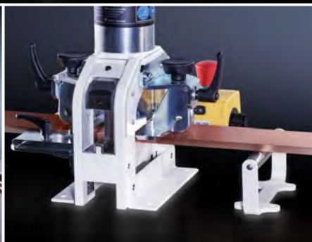
Cutting a busbar to length
