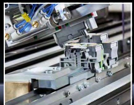
Automated terminal block assembly and labelling with a laser marking system
