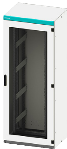
Data cubicles • IP40 • Glass door at front • Section door at rear • Roof with cable entry • 19" fixed-mounted
