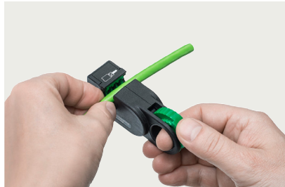
Cut the cable end with the FastConnect stripping tool
