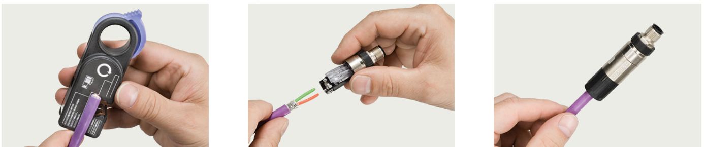
Stripping and assembly with M12 plug-in connector
