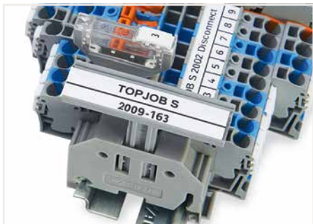
Height-adjustable group marker carrier (2009-163); suitable for WMB markers or marking strips (2009-110)
