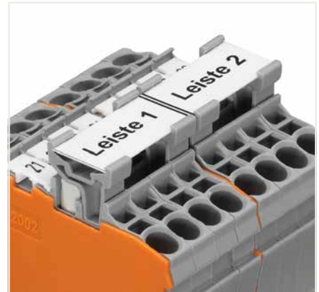
Using marker carriers for marking strips (2002-161) in jumper slots.
